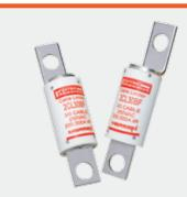
Mersen 2CL Cable Protectors are special purpose limiters which are crimped or bolted to cables or terminals to clear and isolate faults quickly, increasing the reliability of service entrance and distribution runs. They are 250VAC current limiting with a 200,000A interrupting rating, yet will carry low cable overloads which are handled by standard protective devices. These cable protectors are rated for both copper and aluminum cabling per their corresponding cable size.
